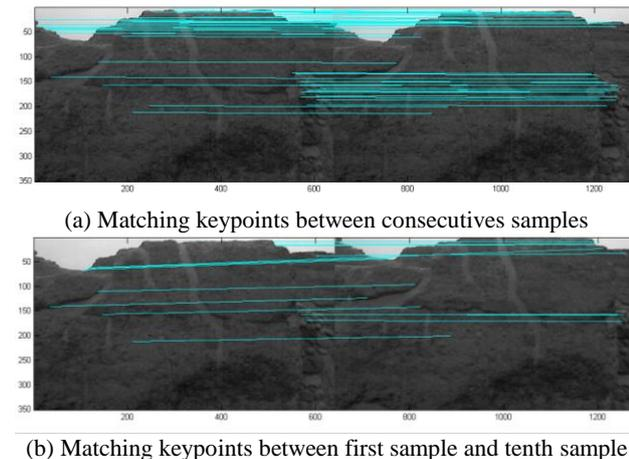
Figure 5: Matching keypoints linked with a light blue bar. In (a) there are 63 keypoints and in (b) just 17.
