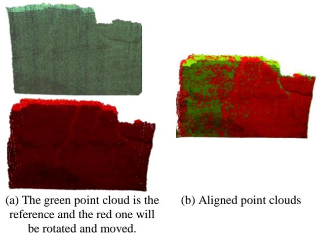
Figure 7: The point clouds (a) will be aligned using  $R$  y  $T$  obtained after applying SURF. The result is shown in (b).
