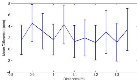
Figure 3: Accuracy error between the Kinect (data being evaluated) and NextEngine Laser Scanner HD (ground truth) for each distance.
