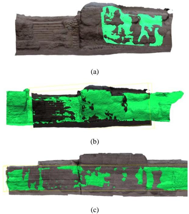
Figure 11: 3D reconstructions alignment of photogrammetry (color) and Kinect (green). Zone 1 of the Inca Path in (a) and (b) and zone 2 (c).
