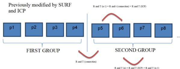
Figure 9: Accumulative process of operating with  $R$  and  $T$  for every point cloud.
