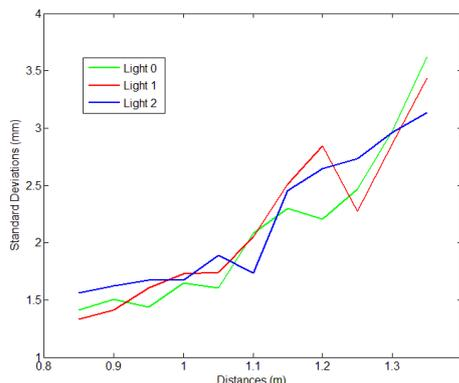
Figure 2: Precision error (standard deviation) versus distances at which the samples were taken.
