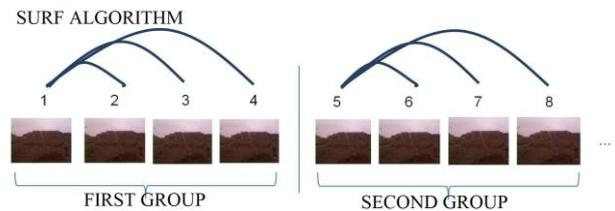
Figure 6: SURF algorithm applied to method group of consecutive color images. All the samples within a group are compared with the first sample of the group.
