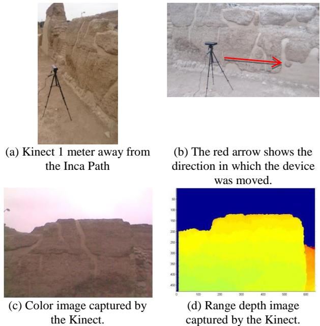
Figure 4: Kinect positioning next to the archaeological site. As the acquisition starts, the device will be manually moved (b) and the captured data will be a set of color images and a range depth images.
