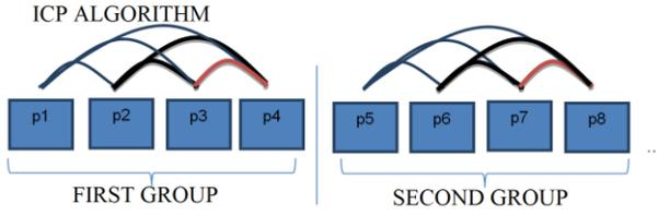
Figure 8: ICP algorithm is applied in a combinatory fashion within each group. For a group of 4 samples, the ICP algorithm is used 6 times.
