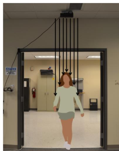
Illustration of the Kinect sensor located on a doorway sensing depth
