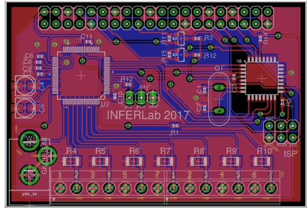
**Figure 1: Metering shield board CAD.**
